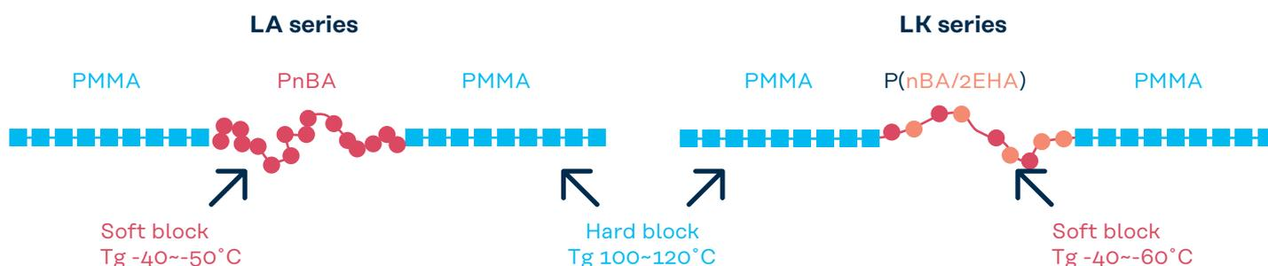
By forming PMMA as the hard block(s) and poly (n-butyl acrylate) or a poly (n-butyl acrylate/2-ethylhexyl acrylate) as the soft block, KURARITY™ exhibits elastomer properties at temperatures lower than Tg of PMMA.
