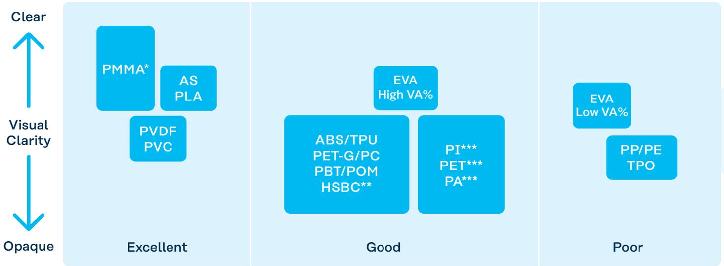
\* Mixing with lower MVR(MFR) MMA causes opaque appearance.
