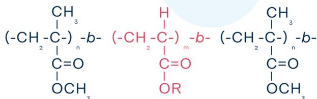
Kuraray leads the world in producing this novel acrylic block copolymer using its unique living anionic polymerization technology. Various type acrylates can be copolymerized as A-B-A type block copolymer.
