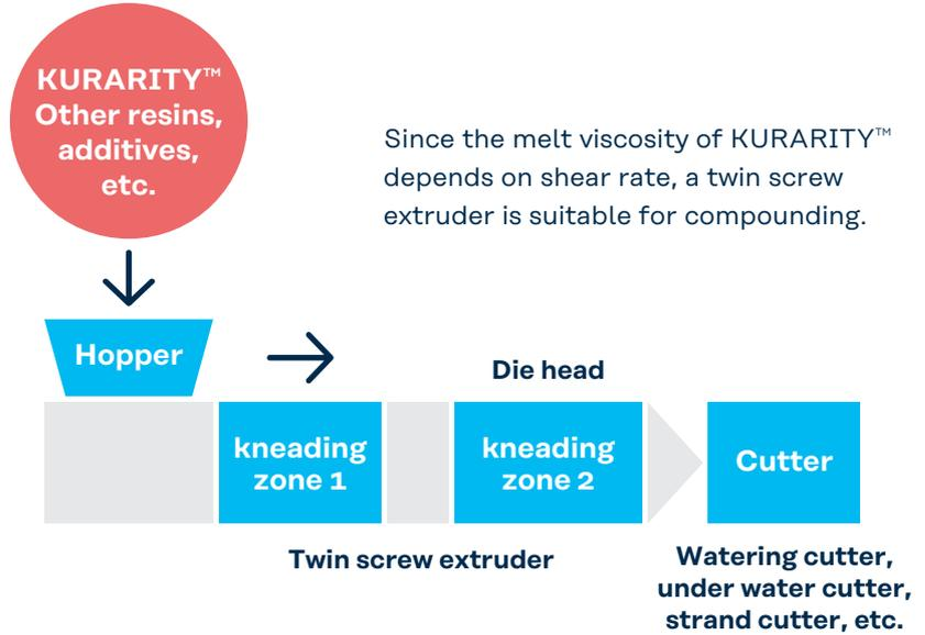
Since the melt viscosity of KURARITY™ depends on shear rate, a twin screw extruder is suitable for compounding.
