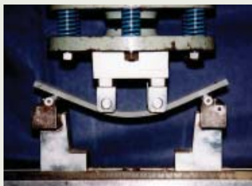
Testing the flexibility of engineered concrete (more flexible and harder to break than older concretes)
